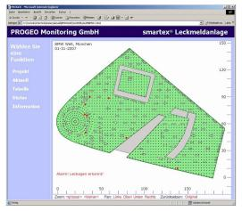
During construction of the BMW World Center in Munich, dozens of areas where leaks had occurred were pinpointed by Smartex MX and repaired before acceptance by the owner
